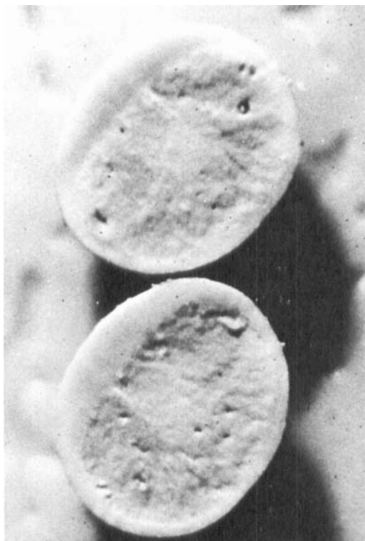
Fig. 4. Cross section of crosslinked polyethylene beads, showing porosity.
